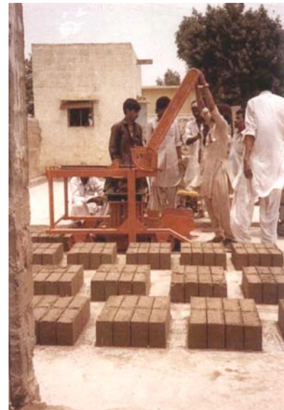
36. Mechanized block making at upgraded thallas.
